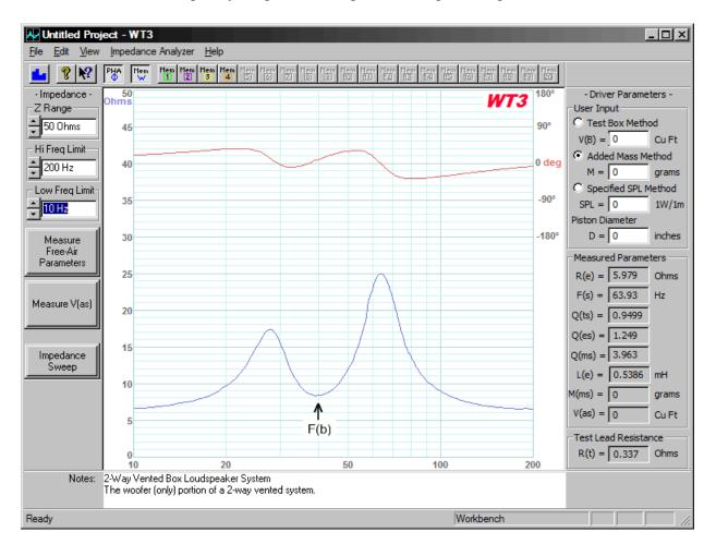
At this screen we can determine that F(b), the tuning frequency of the vented box, is approximately 40 Hz by locating the impedance minimum between the two peaks and reading the frequency where the minimum occurs. The closely zoomed view makes it easier to read the frequency from the scale below.
